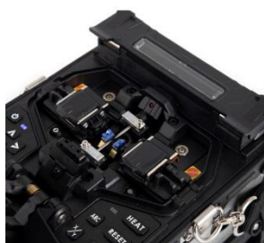
Precise structural design Core to core alignment
