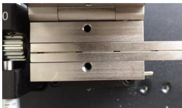
Different fiber holder adapters for different cladding diameter fibers
